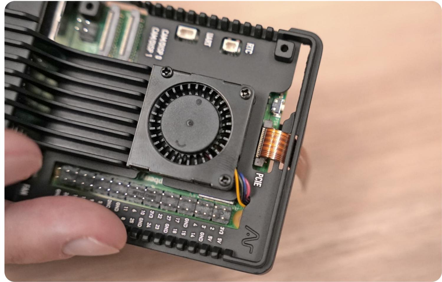
**4.1** The PCIe flat ribbon cable should be threaded through the hole in the case, as shown in the picture
